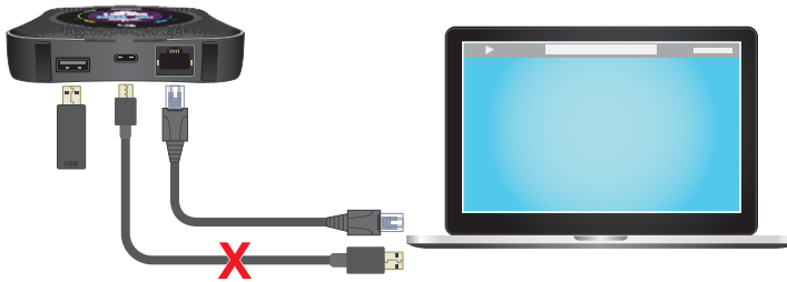
Figure 7. Tethered access is not supported during Ethernet offloading
