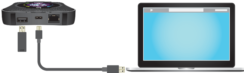
Figure 9. USB storage and tethering connections
